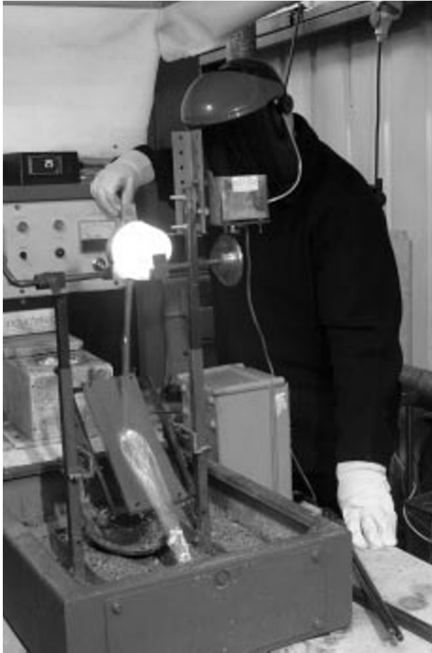
15.2 A fabric being tested to BS EN 373:1993 (courtesy of BTTG Fire Testing Laboratory, Altrincham, UK).
