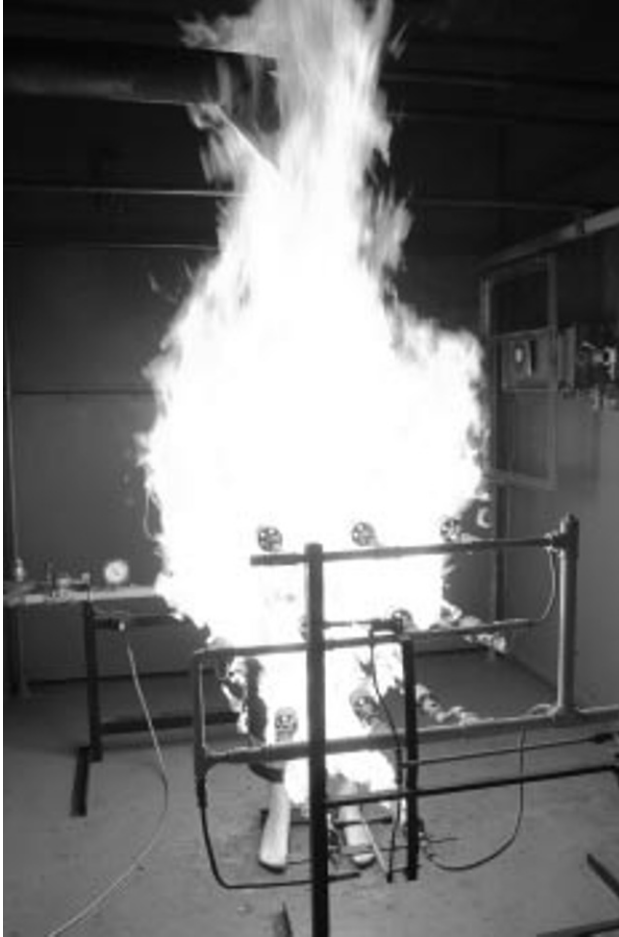
15.3 The BTTG RALPH burner flames at 80 \text{ kWm}^{-2} heat flux engulfing the instrumented manikin (courtesy of BTTG Fire Laboratory, Altrincham, UK).
